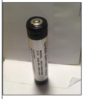
18650 lithium-ion batteries are charged up to 4.2V and down to between 2V and 3V depending on the cell's specification for cut-off voltage.
