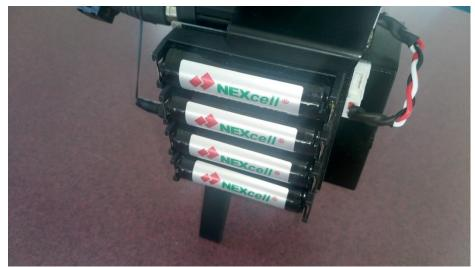
This triples the current battery capacity, providing an increase from approx. 8 hours detecting to approx. 20-22 hours.
