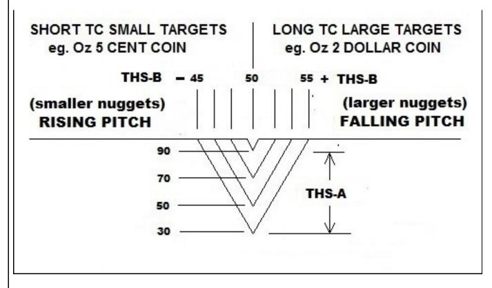
This is how the QED can be set up right on the edge of max performance, either looking for small stuff (biased very low) or looking for bigger stuff (high bias), or at NULL using THS-A (high) looking for any targets.
