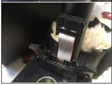
The screen box is connected to the main control box via a connector situated at the top of the front panel of the main control box, directly under the shaft (as per the photo to the left).
